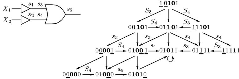
Fig. 2. Circuit  $C_2$  and its binary analysis
